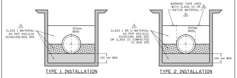
TYPE 1 INSTALLATION REQUIRES THAT THE MATERIAL, DENSITY AND METHOD OF INSTALLATION BE CERTIFIED BY PROFESSIONAL ENGINEER.
