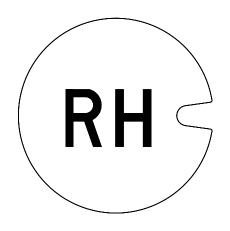
INDICATES VALVE TURNS RIGHT HAND TO OPEN (CLOCKWISE)
