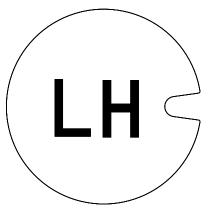
INDICATES VALVE TURNS LEFT HAND TO OPEN (COUNTER-CLOCKWISE)
