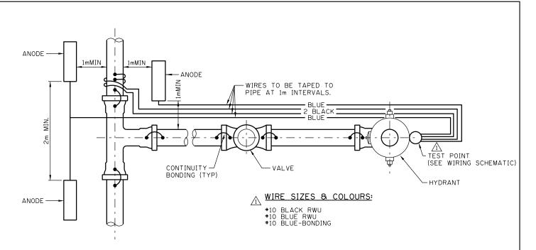
WIRING SCHEMATIC & ANODE INSTALLATION TYPICAL FOR A TEST POINT
