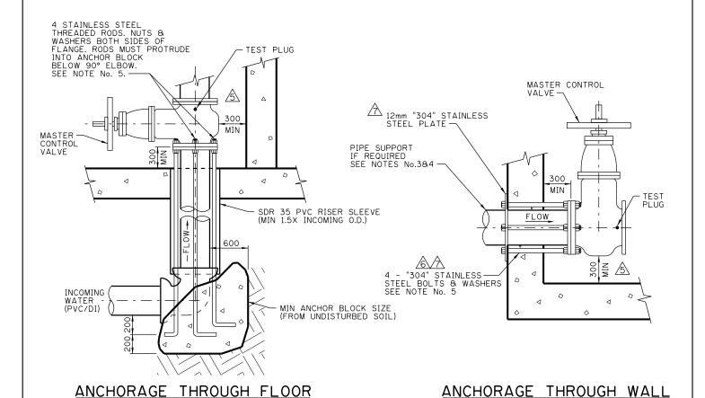
\* BURIED DUCTILE IRON PIPE SHALL BE WRAPPED AS PER 505.03.00 AND PROTECTED WITH A 14.5 KG MAG. ANODE
