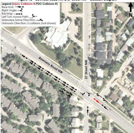
Figure 12 - Bowness Road NW & 37 Street NW - Collision Diagram
