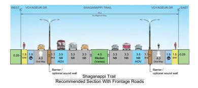
Voyageur Drive will be converted from a two-way configuration to a one-way street to accommodate for the six-lane configuration and to retain street parking and driveway access for residents along Voyageur Drive.
