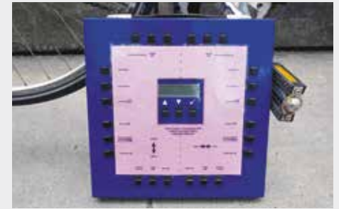
Handheld electronic counter used for manual data collection.
