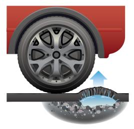
Water freezes and expands, causing the road surface to rise. This is typically called frost heaving.
