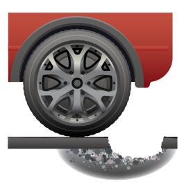
As cars drive over the asphalt, the weight of the vehicles collapse the surface into the void formed by the melted ice. This causes the pothole to form.
