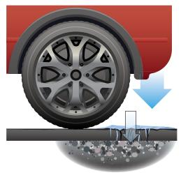
Water seeps through cracks in the asphalt and pools on top of the frozen soil beneath the road surface.
