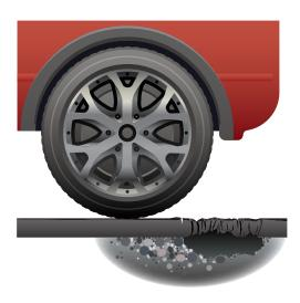
The ice melts leaving a void beneath the asphalt.
