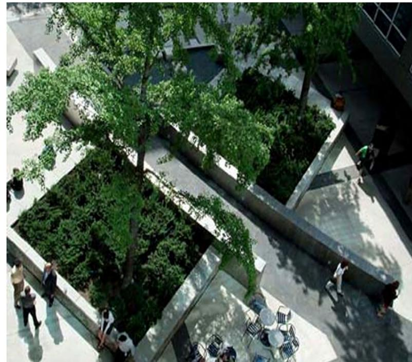
Large tree openings allow more water, oxygen and unobstructed growing medium for trees to develop. Open planter systems also allow fairly free access to maintain utilities within the root zones of trees. Repairs of curbs or retaining walls around the planting zones become conveniently accessible.
